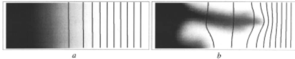
Fig. 4. Results of modeling of displacement for different values of the flow rate [a) Q = 4.8 \cdot 10^{-6} \text{ m}^2/\text{sec} ( \text{Pe} = 17 ) and b) 4.8 \cdot 10^{-5} \text{ m}^2/\text{sec} ( \text{Pe} = 170 )] and the following modeling conditions: T_{\text{in}} = 60^\circ\text{C} , c_s = 1.4 \cdot 10^5 \text{ J}/(\text{m}^3 \cdot \text{K}) , M = 38 , R = 1.9 , and \eta = 0.4 .
